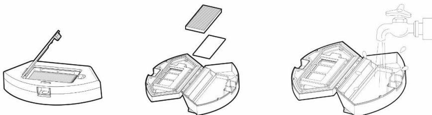
Clean the HEPA filter regularly according to the degree of its contamination, at least once a week, with a dust brush or vacuum it with a standard vacuum cleaner.
