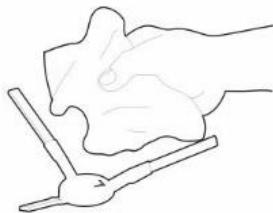
Check both side cleaning brushes together with the air intake opening according to the intensity of the contamination, at least once a week, and remove tangled hairs and other dirt.
