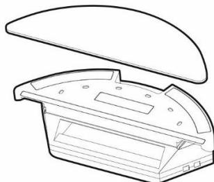
Install the blue mop cloth on the bottom of the water tank. Slightly moisten the mop cloth with water for faster and smoother water wiping.
