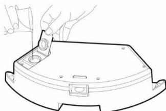
Open the plastic cap and collect water into the water tank. Only add water to the wiping container after removing the container from the vacuum cleaner. A slight leak of residual water may occur when handling the water tank. In this case, wipe the spilled area immediately with a dry cloth.
