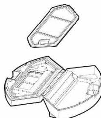
Press the release button to remove the dust tank and empty the dirt into the waste bin.
