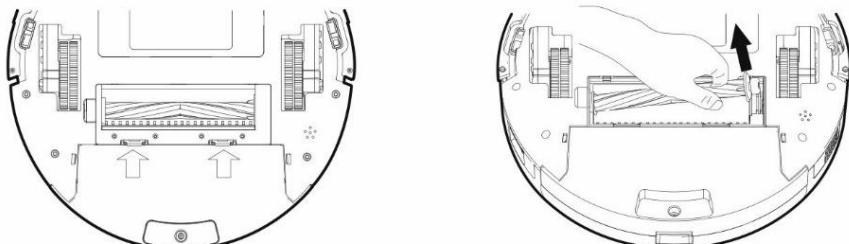
To remove the main central cleaning brush, press both tabs on the brush cover. Use a cleaning tool to remove hair entangled in the main central brush. Keep the central cleaning brush free of much hair, dust, cotton, etc.
